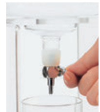
Use the faucet to adjust dripping rate.
